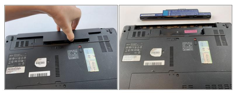
• Remove the battery pack via the indentation at the top of the battery in between the two switches.
