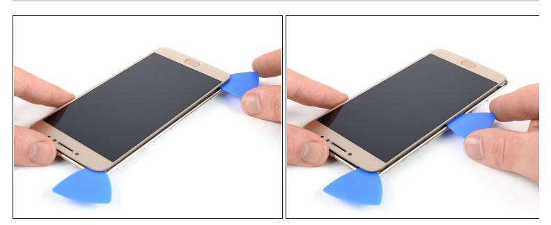
• Repeat the previous heating and cutting procedure on the left edge of the phone to cut the remaining adhesive.
