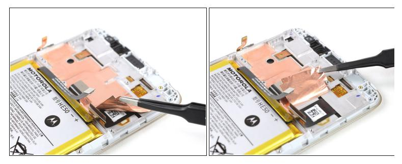
• Use a pair of tweezers to peel the copper tape from the right edge until the display flex cable underneath is fully exposed.
