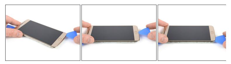
• Slide the opening pick along the bottom edge of the phone and cut the adhesive.
