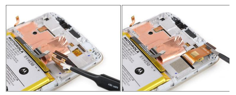
• Use a pair of tweezers to carefully peel the display flex cable off of the midframe.
