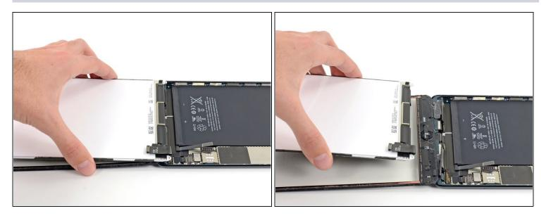
• Lift and remove the LCD from the iPad Mini.
