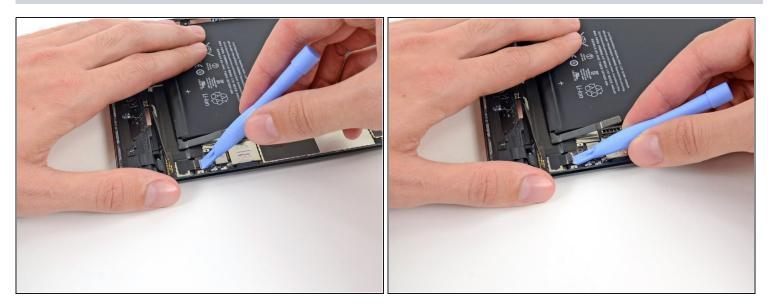
A Be very careful to pry evenly on the digitizer connector, and not on the socket at all. The socket and connector are very delicate and if you damage either, your digitizer won't work.
