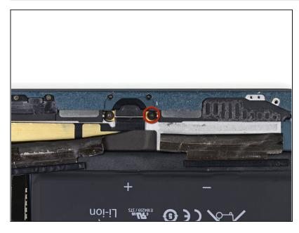
• Remove the single 1.4 mm Phillips #00 screw securing the left speaker to the rear case.
