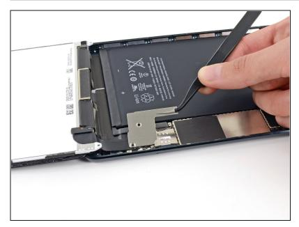
Use a pair of tweezers to grasp and remove the connector shield from the iPad.
