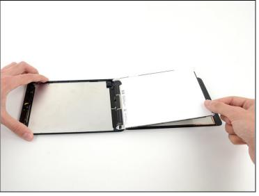
• Flip the LCD over and rest it on top of the front panel glass.
