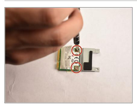
Flip the wireless card over and unscrew the two screws shown in the picture, detaching the wireless card from the plate.
