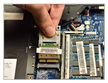
Pull the wireless card out of its socket.
