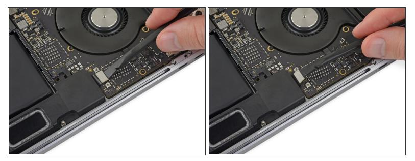
• Disconnect the Touch Bar display cable by prying its connector straight up from the logic board.
