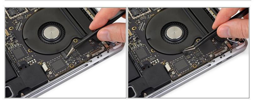
Peel up any tape covering the microphone cable connector socket.
