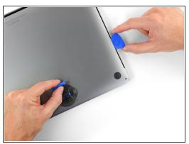
Repeat the previous step on the other side, using an opening pick to to release the second clip.
