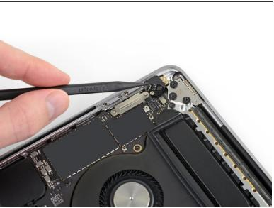
Disconnect the headphone jack flex connector by prying it straight up from the logic board.
