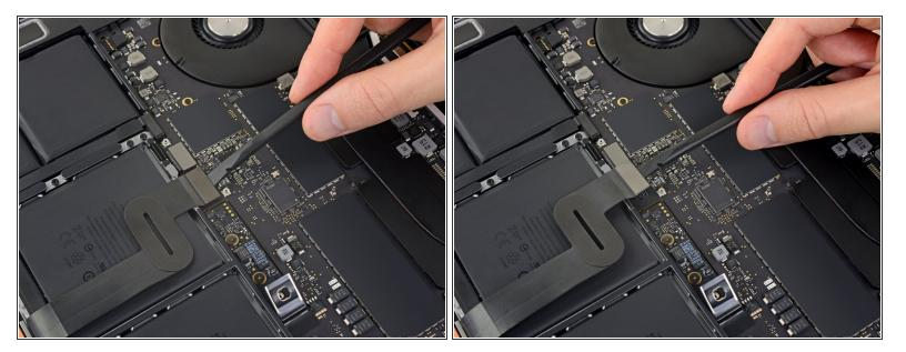
Use a spudger to disconnect the trackpad cable by prying its connector straight up from the logic board.
