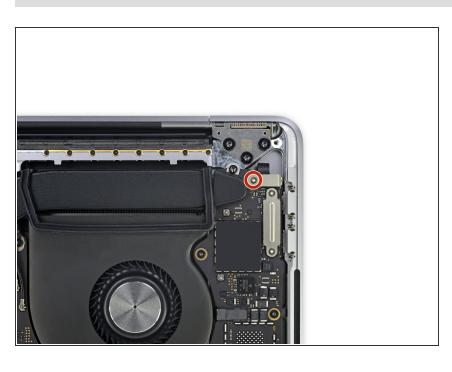
Using a T3 Torx driver, remove the 1.3 mm screw securing the cover bracket for the Touch Bar digitizer connector.
