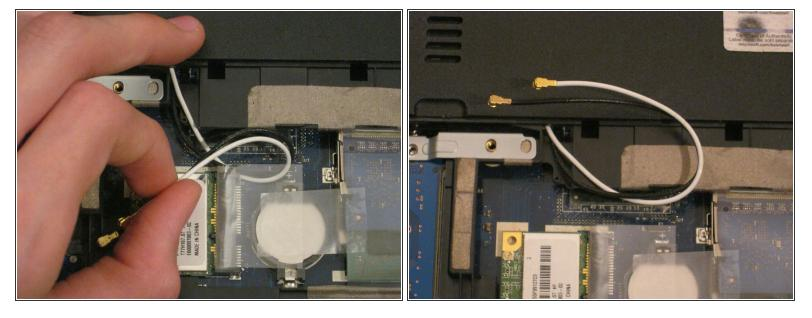
(i) You may find it useful to pull the antenna cables out from under the plastic retaining clip so you can move them out of the way while you work.
