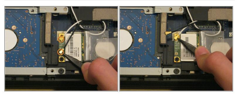
Use the pointy end of a spudger to remove the antenna connectors from the WLAN card.
