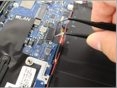
Pull the battery cable connector towards the battery to disconnect it from its socket.
