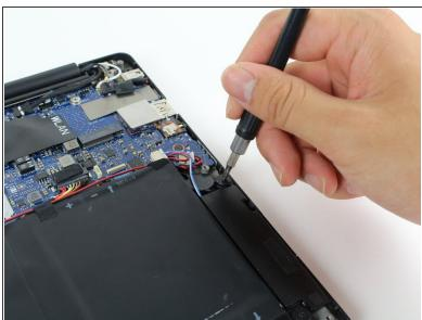
Remove the four 3 mm Phillips #0 screws located on each corner of the battery.
