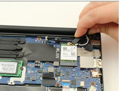
Pop the coaxial antenna cables up from the wireless card with the flat end of the spudger.
