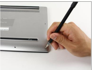
Remove the eight 4 mm T5 Torx screws from the bottom cover.
