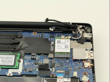
• Use your fingers to remove the sliding camera connector out from the motherboard.
