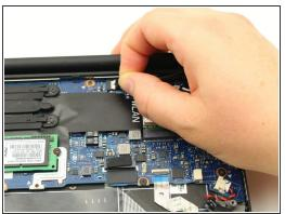
Pull the sliding touchscreen connector gently to the right and out of the motherboard.
