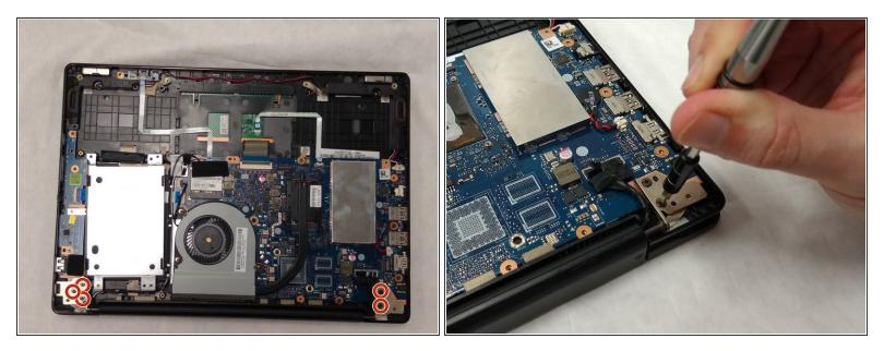
• Use a Phillips #00 screw driver to remove the five 10mm screws at the hinges.
