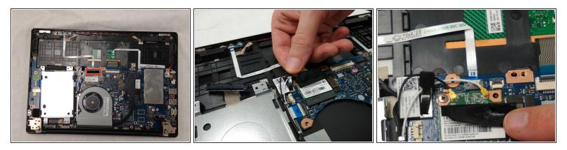
• Peel back the tape and remove the two connectors.
