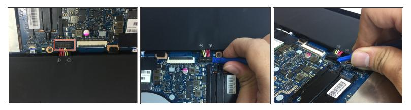
• Gently wedge a plastic opening tool under the connector.
