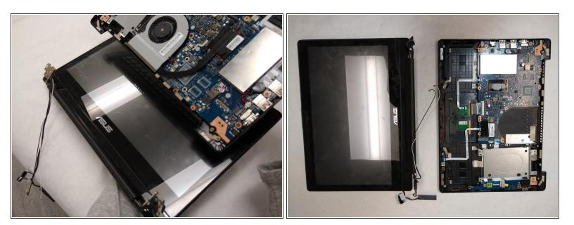
• Carefully remove the display from the rest of the laptop.
