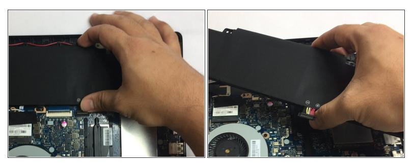
• Once the screws and connector are removed, simply pull out the battery from its place.
