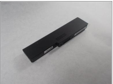
Remove the battery from the battery compartment.
