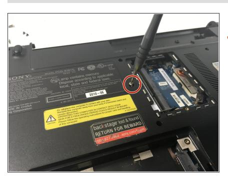
Use a JIS #0 screwdriver to remove the 4mm screw from its place.
