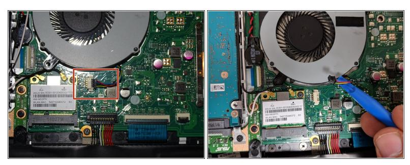
• Carefully unplug the fan cable from the motherboard using a spudger or plastic opening tool.
