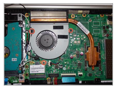
Remove three 5mm Phillips #1 screws that are holding the fan in place.
