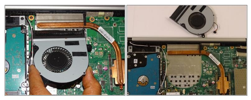
Carefully use your hands to remove the fan by pulling it from the heatsink housing.
