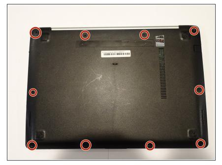
Remove all ten 6mm Phillips #1 screws from the bottom of the computer chassis.
