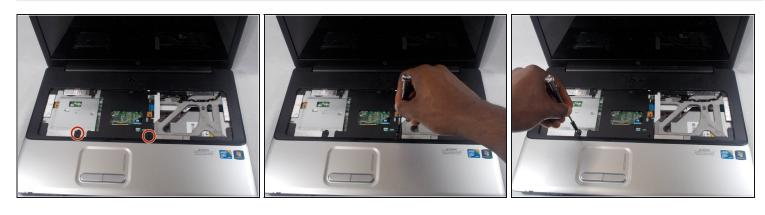
Remove the circled screws to release the bezel from the faceplate.
