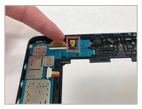
Locate the camera at the top of the device.
