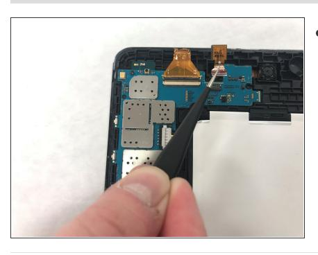
Remove the front camera and replace it with the new part.
