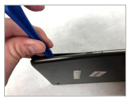
Pry along the edge of the Samsung Galaxy Tab A 9.7 with an iFixit opening tool.
