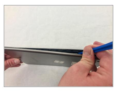
Remove one of the opening tools and begin to go around the device with the other one until the back cover pops off.
