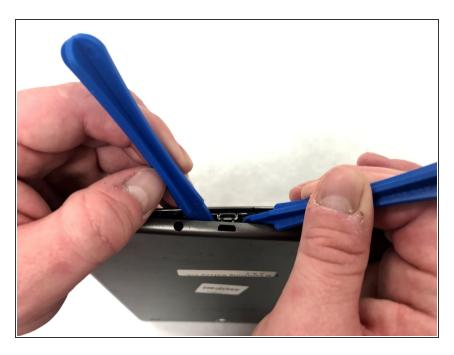
Insert a second iFixit opening tool along the edge and begin to pry open the back cover a little with each one.
