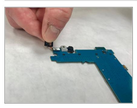
Pull off the rear camera on the back of the motherboard and replace.
