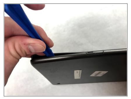
Pry along the edge of the Samsung Galaxy Tab A 9.7 with an iFixit opening tool.
