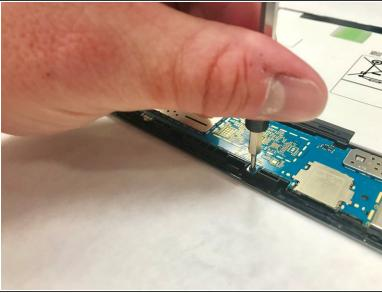
• Remove five 2.8 mm screws using the Phillips #000 screwdriver.
