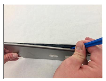
Remove one of the iFixit opening tools and begin to go around the device with the other one until the back cover pops off.
