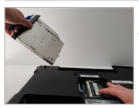
Using an iFixit opening tool, carefully pry the disk drive away from the device.
