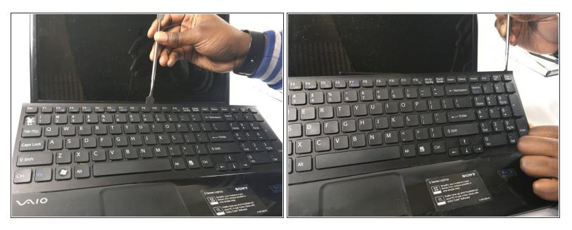
Continue lifting up and moving down starting on the left side of the keyboard moving towards the right side of the computer.
