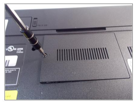
Remove the single screw holding the panel in place using the JIS #0 screwdriver.
