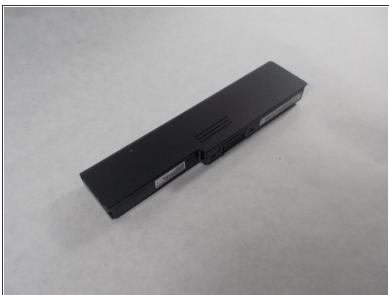
Remove the battery from the battery compartment.
