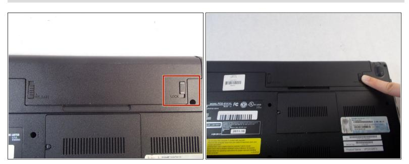
Slide the lock switch down until you hear a click to unlock the battery.
