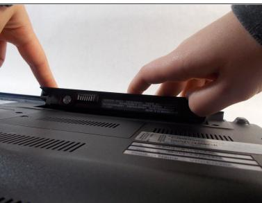
Slide the release slider up and simultaneously push the battery upwards away from the device until it falls out of place.
