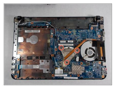
Remove the three 7mm screws attached to the fan using the JIS #0 screwdriver.
