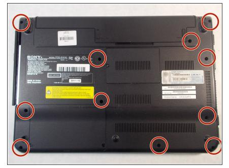
Remove the remaining eleven 7mm screws from back panel using the JIS #0 screwdriver.
