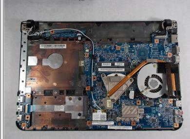
Remove the back panel from the device.
