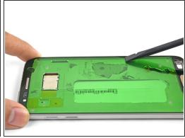
Once the adhesive is aligned on the frame, run the flat end of a spudger around the perimeter of the adhesive to press it into place. You can also use your fingers.
