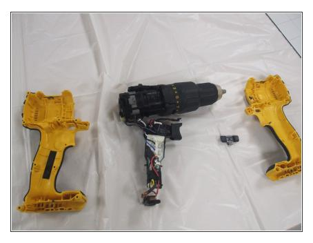
Remove the drill mechanism from the shell.
