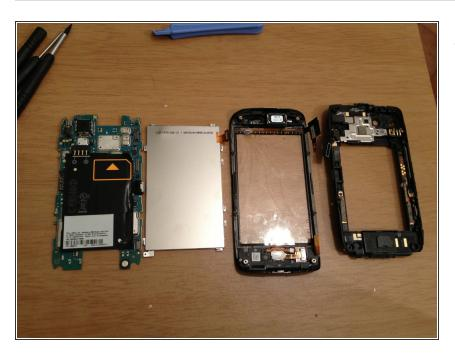
Once the LCD is removed, the handset disassembled.
