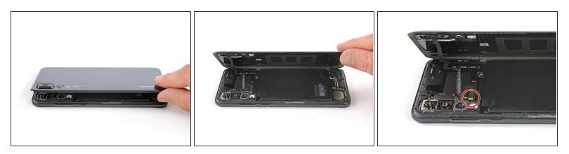
• Carefully lift the rear glass until you can reach the connector of the proximity sensor flex cable next to the rear camera assembly.
