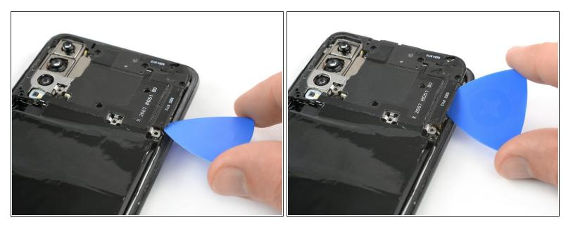
Repeat the previous process on the right side and twist the opening pick to pry up the motherboard cover.
