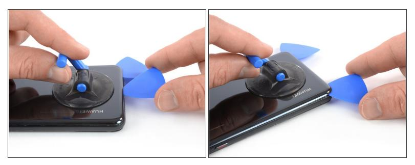
Insert a second opening pick and slide it to the bottom left corner. Leave it there to prevent the adhesive from resealing.
