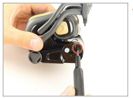
Unscrew the two body screws beneath the wheel using the same screwdriver.
