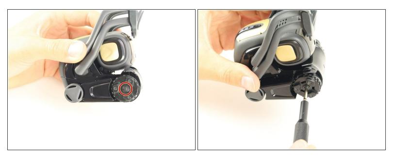
• Unscrew the wheel with the Phillips #00 screwdriver and gently remove it.
