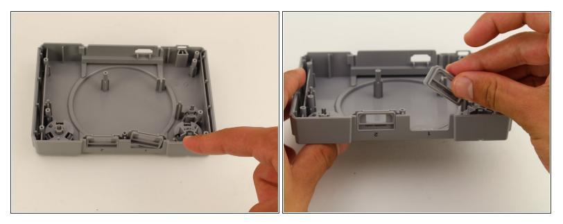
• Identify the damaged or faulty controller port and simply use your fingers to remove.
