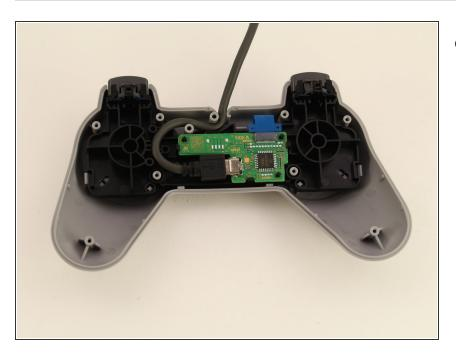
You will notice that the controller cord is plugged into a Micro USB port on the controller motherboard.
