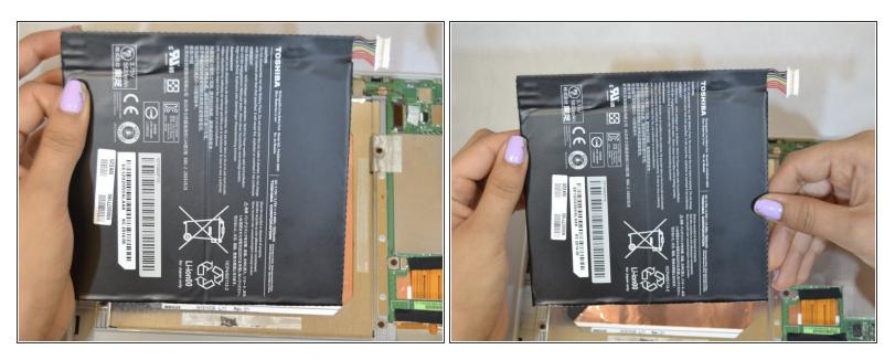
• Remove the battery from the compartment.
