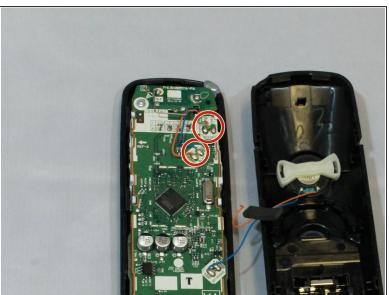
Identify damaged or loose wires. If loose, adjust till properly placed. If damaged, solder the new wire(s) to the mother board or desired location.
