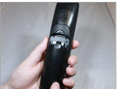
Remove the battery cover by sliding the cover piece down
