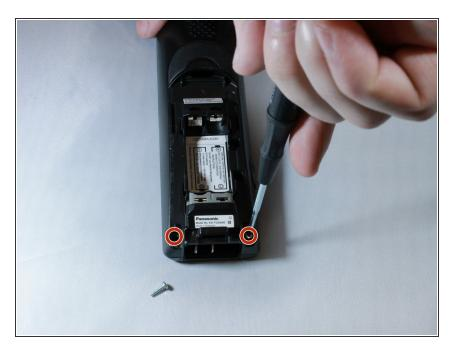
Unscrew the two screw at the bottom of the device.
