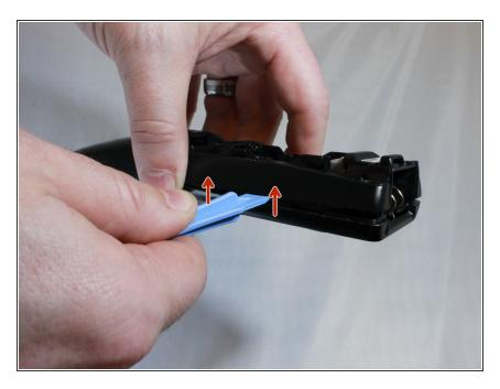
Using the iFixit opening tool, pry open the back of the phone.
