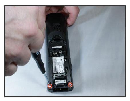
In order to remove the back of the phone, unscrew the two screws at the bottom corners on the back of the phone.
