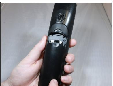
Remove the battery cover by sliding the cover piece down
