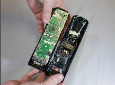
In order to remove the back of the phone, pry the back open by inserting the iFixit Opening tool in the space between the front and back of the phone.
