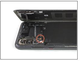
Carefully lift the rear glass until you can reach the connector of the proximity sensor flex cable next to the rear camera assembly.
