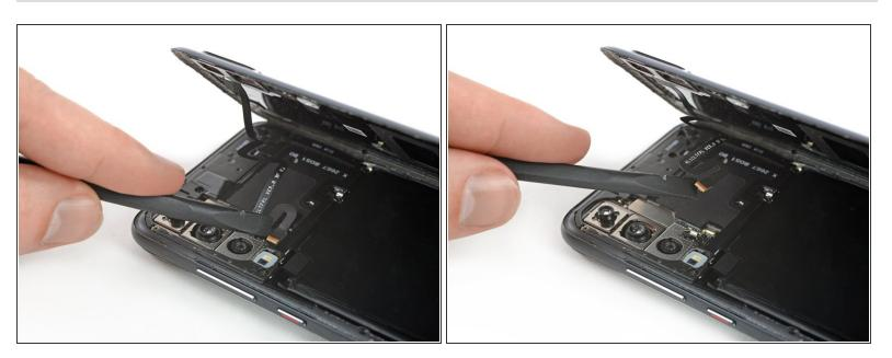
Use the flat end of a spudger to pry up and disconnect the proximity sensor flex cable.
