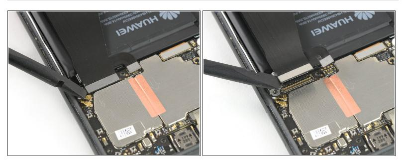
Use the flat end of a spudger to pry up and disconnect the upper end of the interconnect and charging port flex cable from the motherboard.
