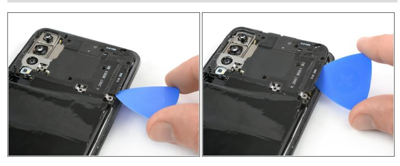
Repeat the previous process on the right side and twist the opening pick to pry up the motherboard cover.
