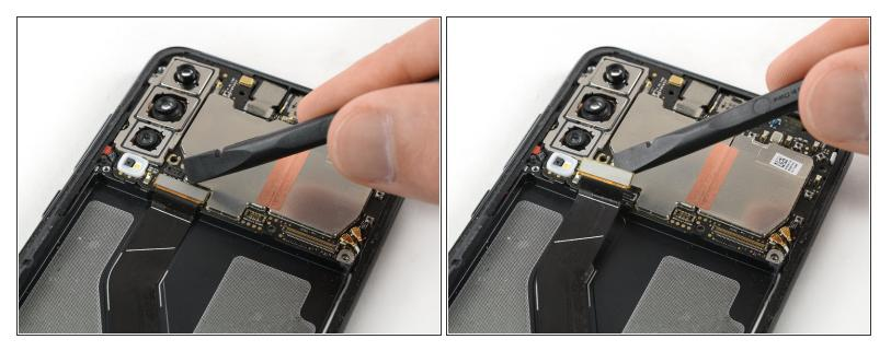
Use the flat end of a spudger to pry up and disconnect the display flex cable at the bottom left of the motherboard.
