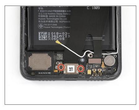
Remove the two Phillips #00 screws (3.4 mm length) on both sides of the USB C port.
