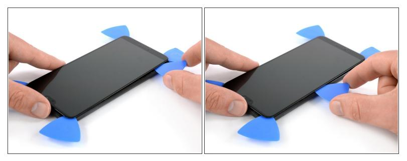
Insert a fifth opening pick and slide it along the left edge of the phone to cut the remaining adhesive.
