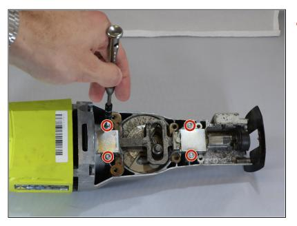
Unscrew the four T5 Torx screws that hold the assembly bar in place.
