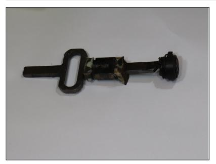
• Lift the assembly bar up and out of the chassis.
