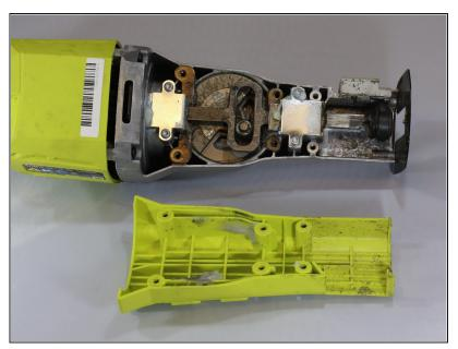
• Remove the backside panel.
