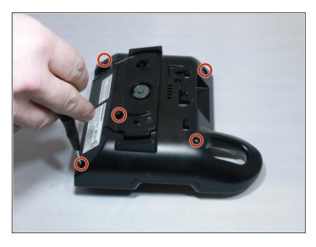
• Use a Phillips #0 screwdriver to remove five screws from the back cover.
