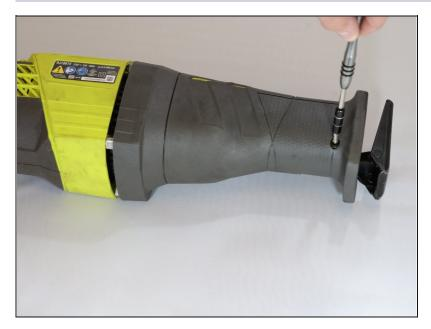
Use a Torx T5 screwdriver to remove the single 8 mm screw securing the shoe.
