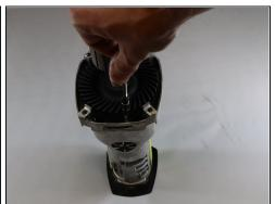
• Use a Torx T5 screwdriver to remove the four screws attaching the motor to the gear case.
