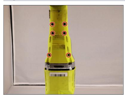
Use a Torx T5 screwdriver to remove the six screws on the underside of the device.
