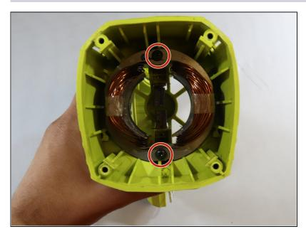
Use a Torx T5 screwdriver to remove the two screws inside the motor housing of the handle.
