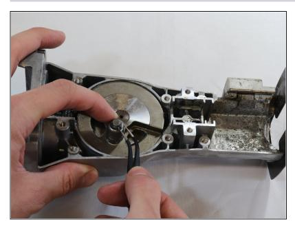
• Insert needle nose pliers to remove the retaining pin at the top of the bearing.
