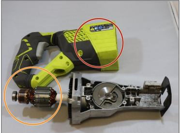
• After following prerequisite guides to get to the presented step, remove motor assembly from back housing.
