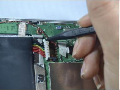
Use plastic spudger to remove the attached battery wires by pushing the plastic wire holder from right to left on top and bottom part of plastic holder.
