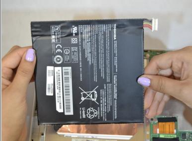
Remove the battery from the compartment.
