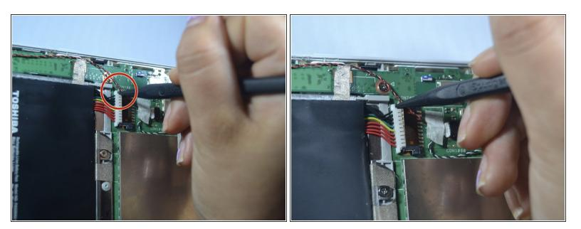
• Use plastic spudger to remove the attached battery wires by pushing the plastic wire holder from right to left on top and bottom part of plastic holder.
