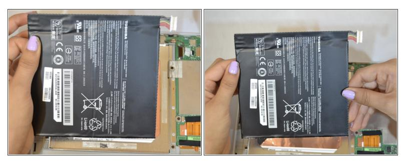
• Remove the battery from the compartment.
