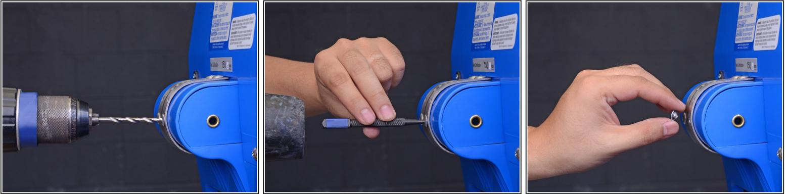
**i** This step shows how to drill a rivet out.
