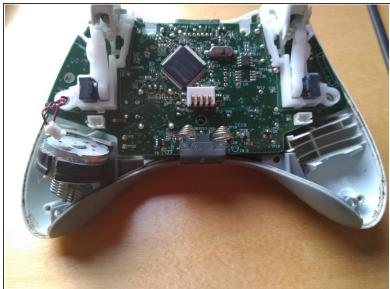
Detach the vibration motor cable from the PCB.
