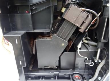
The cover over the brewing unit is only lightly gripped. Lift it out.
