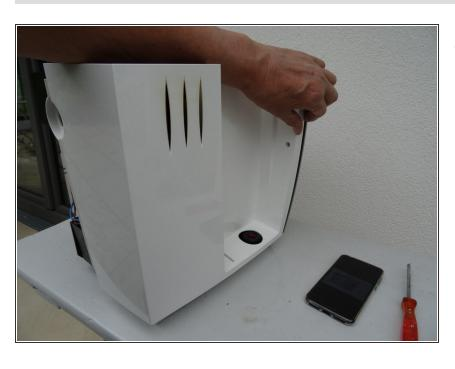
Pull the left side panel slightly towards the back and remove it.
