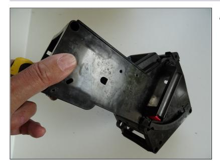
• Remove the brewing unit from the device.
