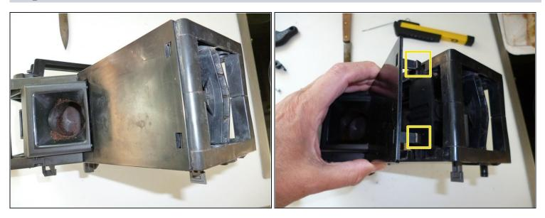
• Unclip the upper protection panel, then remove it by lifting it up.
