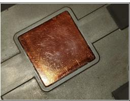
Repeat that process on the heatsink. This will allow for even distribution of the thermal paste to fill properly.
