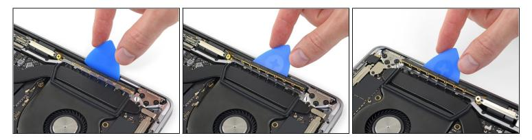
• Use an opening pick to pry up the antenna assembly and separate it from the MacBook Pro.
