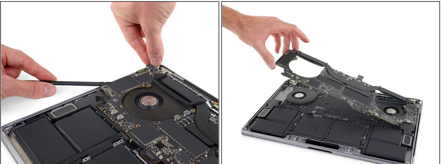
ⓘ The logic board assembly is a tight fit, but you can make it easier to remove by inserting a spudger under the left edge and levering it up slightly.
