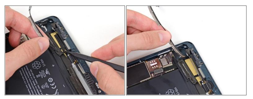
• Use the tip of the spudger to pry the antenna cable tape up from behind the right speaker as well.
