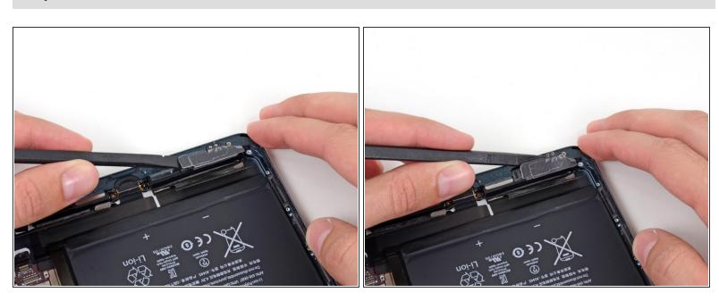
Use the flat end of a spudger to loosen the foam adhesive securing the Wi-Fi antenna to the left speaker.
