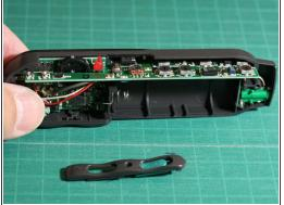
Carefully remove the bezel around the volume dial power switch and on/off indicator LED. Be careful not to lose the small power button cap which will come loose after removing the bezel
