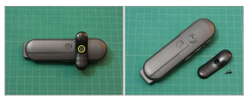
First, remove the screw in the center of the clip using a Phillips #0 screwdriver, and then remove the clip
