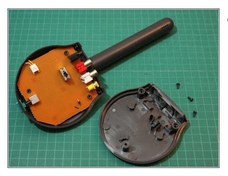
Once the screws are removed, you can lift off the bottom cover.
