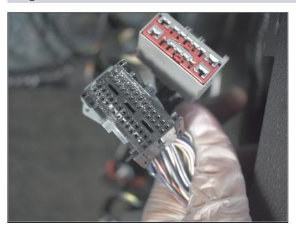
Inspect all connectors for corrosion to indicate where the junction box needs cleaning.
