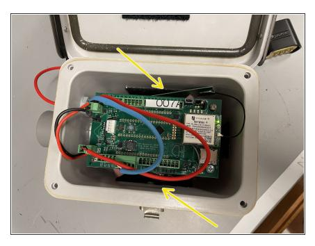
Attach the antenna, and the GPS on the velcro to the closest wall on the inside of the enclosure
