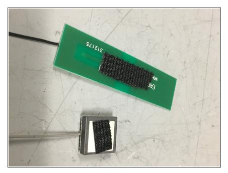
Attach rough-sided velcro on the antenna and GPS as shown in the picture.
