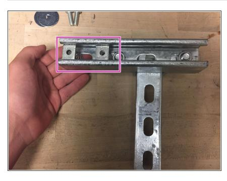
insert the two 5/16" strut channel nuts into the back of the horizontal strut channel as shown
