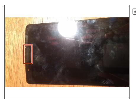
Before reassembly, be sure to transfer the front speaker grille if it is not included with the new screen. If not, carefully push the grille out from the old screen, then reinsert it on the new LCD.
