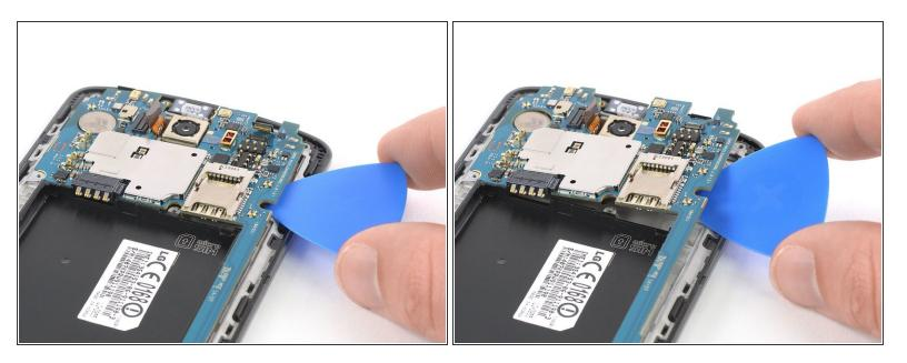
Slide the opening pick under the right edge of the motherboard where the SIM card slot is located and pry it up by rotating the opening pick sideways.
